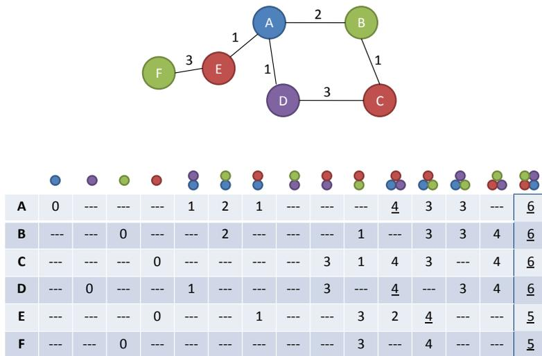
Figure 3.1: A single run of the dynamic programming. Top: a vertex-colored graph with weighted edges. Bottom: The dynamic programming the table. The columns correspond to the possible color subsets, and the rows correspond to the vertices. Each cell  $(v, S)$  contains the score of the maximum-weight tree rooted in  $v$  and colored exactly by  $S$ . For easier tracking of the algorithm, the values in the cells in the stages where there were several trees to choose from are underlined.
