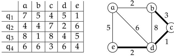
Figure 5.4: Example for PATHWAY QUERY with  $l = 4$  and  $N_{ins} = N_{del} = 1$ . Query sequence is  $q_1, q_2, q_3, q_4$ . Left: vertex match table  $h$ . Right: weighted graph  $G$ . The optimal path is  $P = edcb$  (*bold edges*) with matching  $M : q_1 \mapsto e, q_2 \mapsto d, q_3 \mapsto b, q_4 \mapsto \perp$ . The cost of this solution is  $2 + 1 + 3 + 1 + 2 + 1 = 10$ .
