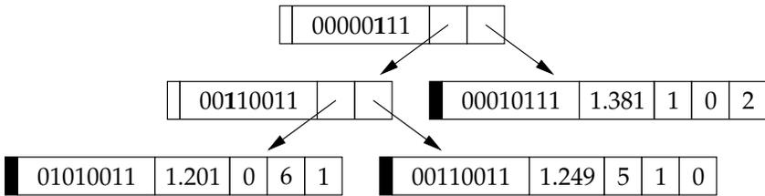
Figure 5.8: Representation of color sets at some node  $u$  with color 4. Inner nodes contain the marker bit (leftmost box), the common suffix (branch bit in bold), and two pointers to children. Leaf nodes contain the marker bit, the color set, the weight, and the vertices of the path.
