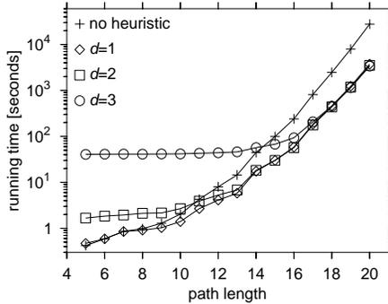
Figure 5.7: Running time comparison with heuristic evaluation functions for different values of  $d$  (seeking the 20 lowest-weight paths in the yeast network of Scott et al. [2006] that differ in at least 30% of participating vertices).
