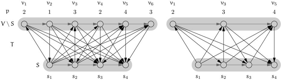
Figure 4.10: Example for the subroutine in Figure 4.8. For clarity, only some of the arcs within the acyclic subtournaments  $T[S]$  and  $T[V \setminus S]$  are shown. Left: Tournament  $T$  after data reduction with  $L = v_1, v_2, v_3, v_4, v_5, v_6$  and  $P = v_2, v_1, v_4, v_3, v_6, v_5$ . A longest common subsequence is  $v_1, v_3, v_5$ , yielding the acyclic graph shown on the right.
